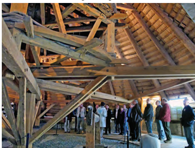
The massive horse windlass, reconstructed from a nearby mine, at the Kutna Hora silver mine
